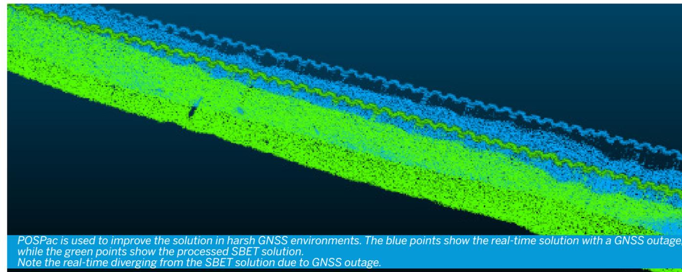
POSPac is used to improve the solution in harsh GNSS environments. The blue points show the real-time solution with a GNSS outage, while the green points show the processed SBET solution. Note the real-time diverging from the SBET solution due to GNSS outage.
