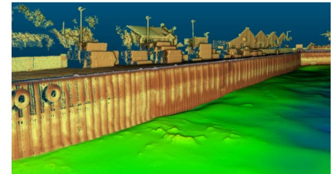
Vessel-mounted LiDAR and Multibeam compliment each other to provide precise data above and below the water line.
